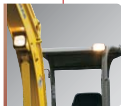
The convenient light arrangement expands the operator's field of view for night work.
