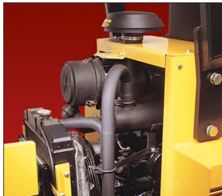
The lift-up cowl provides optimum access for servicing and protects the 58 hp John Deere engine, muffer and other components.
