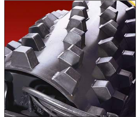
Earth-Crushing Padfoot. Helically placed pads deliver maximum compactive force on cohesive soils. Two pads are always in contact with the soil to give you a smooth, effective roll.
