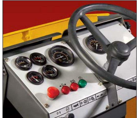
Instrumentation panel provides easy visibility to gauges.
