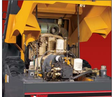
Lift-up fiberglass hood provides maximum access to engine compartment. Pumps and filters, fuel and hydraulic fill caps and all components are easily accessible at rear of compartment. Makes routine servicing fast and easy.
