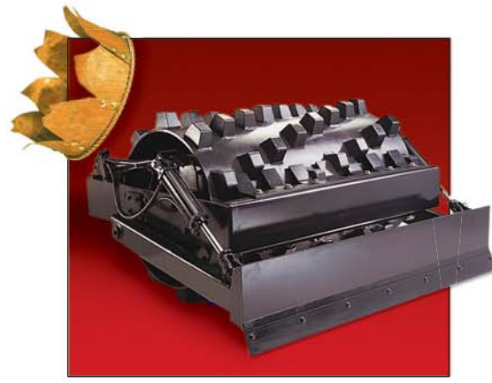
Optional knockdown blade available on padfoot models. Use this blade to grade or to level uneven soil and terrain.
