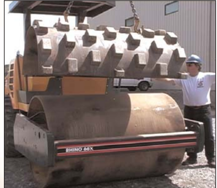
With a Rhino SD66X smooth drum vibratory dirt roller and a padfoot conversion kit you have the versatility of two rollers in one. The conversion kit features drum shells, scrapers, hardware and an anti-spin device. Roller weight with padfoot installed: 18,846 lbs (8,566 kg).
