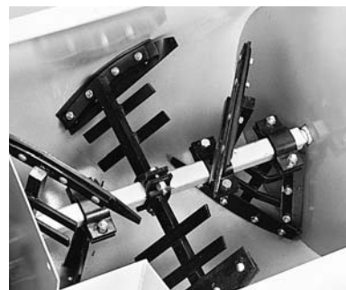
Exclusive, patented Power Blend mixing action gives you fast, thorough blending. Using a unique arrangement of rubber and steel blades on an exclusive paddle configuration. Six paddles rotate in a triple eight mixing action, constantly dividing and recombining the mixture for a smooth uniform mix.
