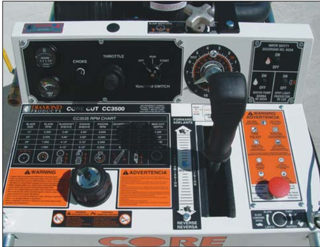
CC3500 Control Panel
